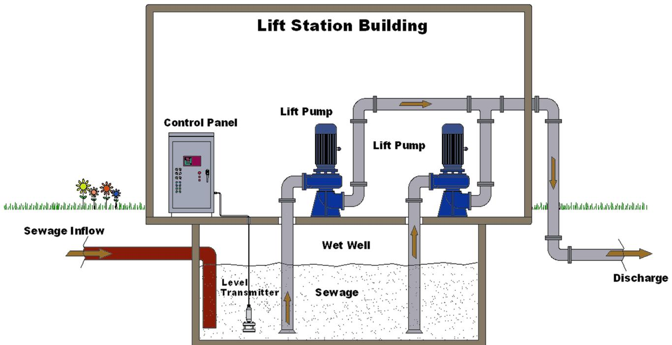
The purpose of the level transmitter is to provide feedback to the pump allowing them to turn on and off when the level reaches a set height. Floats, bubbler systems, radar and ultrasonic are all ways to indicate level. However these methods can have installation difficulties, maintenance issues, high costs or reliability issues due to the environment.
